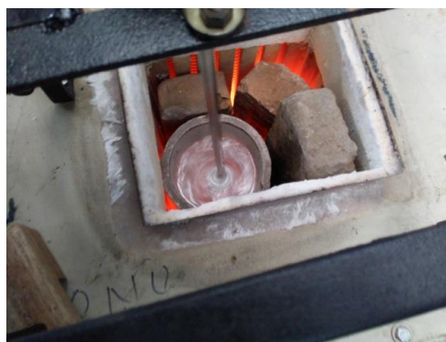
Figure 3: Melting of Al 6061 in muffle furnace
