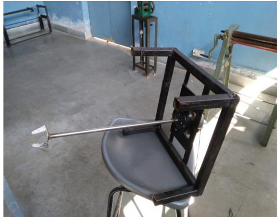
Figure 4: stirrer with Thermocouple.
