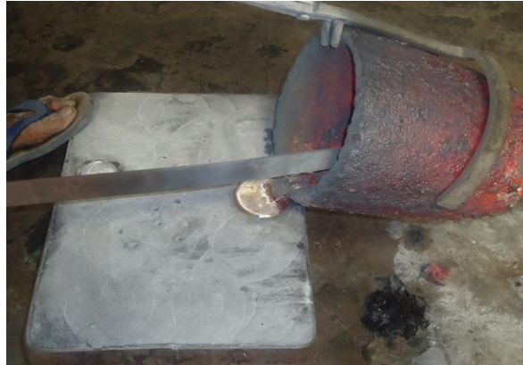
Figure 6: Pouring of molten Al into mould.
