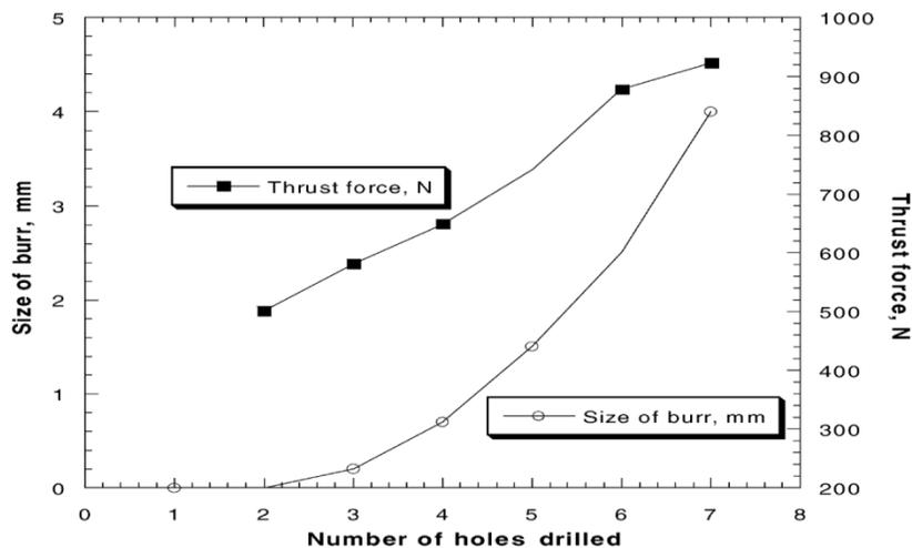
Figure 4 Thrust force and burr size produced with HSS drill while drilling  $(Al_2O_3)p/6061$  (Ramulu, Rao, and Kao, 2002)
