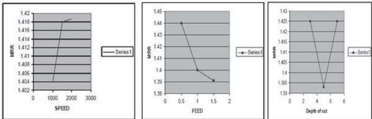
Figure 3 Effects of input parameters on MRR (Tyagi, Chaturvedi, and Vimal, 2012)
