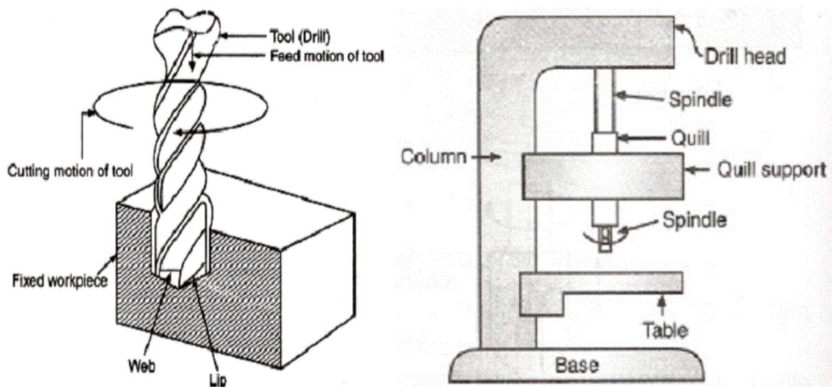
**Figure 1 Basic diagram of drilling operation**
