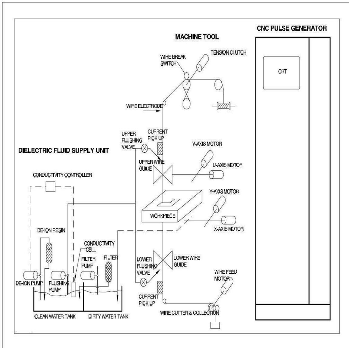
**Figure 1 Set-up of WEDM process**
