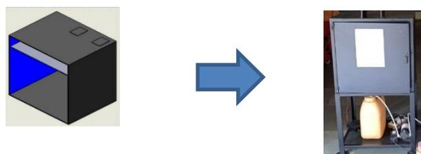
Which is to use UV radiations for sanitization purposes. Comprises paddle operated door mechanism.
