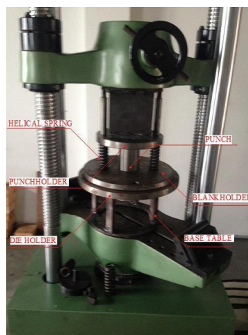
Figure 2. Deep drawing tool setup
