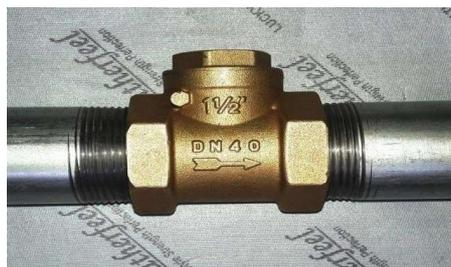
into the exhaust pipe and clogs it. So, in order to sidestep this issue a non return valve is attached. The valve does not let the water flow in both directions and keeps the water trapped in the aqua silencer.
