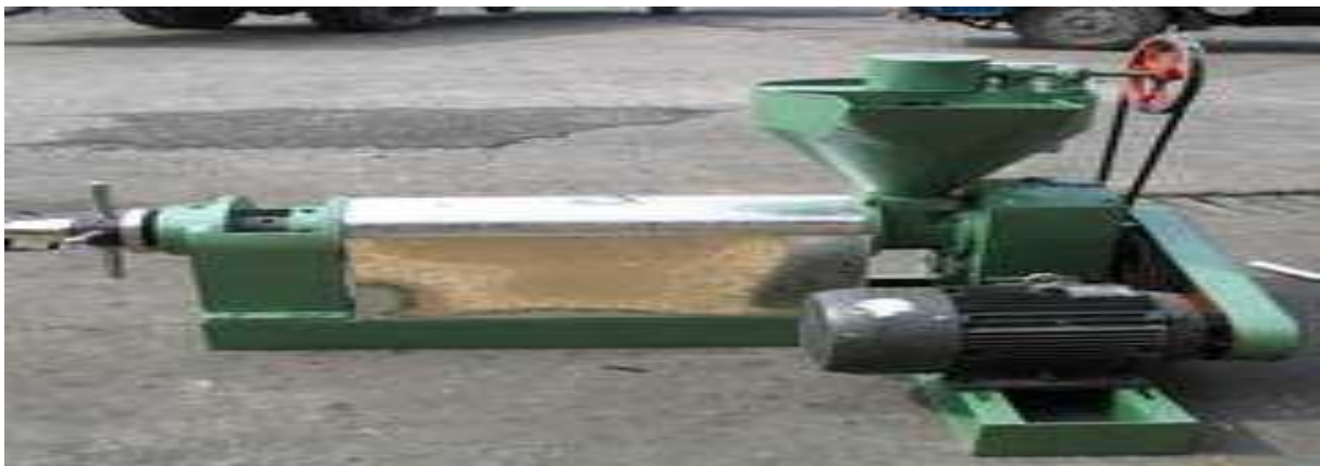
Figure 4. Karabi oil presses in lab
